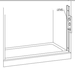
**2.** Remove each wall jamb. Drill 3/16" diameter holes in previously marked walls. (For tiled walls, use a carbide tipped drill bit) Insert plastic wall anchors (#2) into holes. Silicone where the wall meets the curb of the tub/shower to seal behind the bottom of jambs. Set jambs in place and secure to the wall with #8 x 1 ½" SMS screws (#3).
