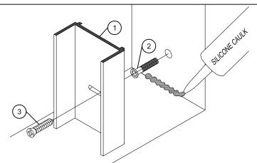
**3.** Cut header (#8) 1/32"-1/16" less than opening width and screw in place with #6 x 3/8" SMS screws (#10).
